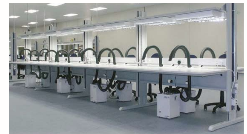
Arm extraction install example below for soldering application:
